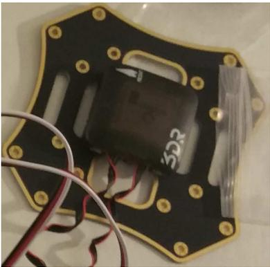
Figure 7: GPS/compass module placement
