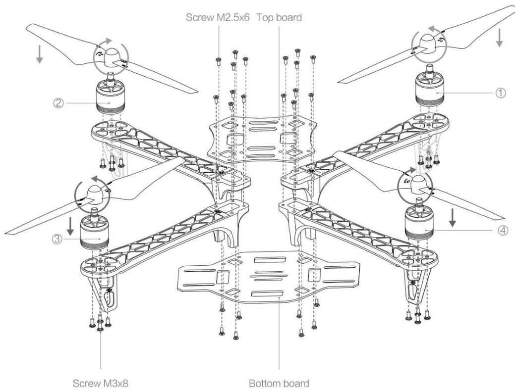
Figure 1: Flamewheel F450 assembly diagram[7]
