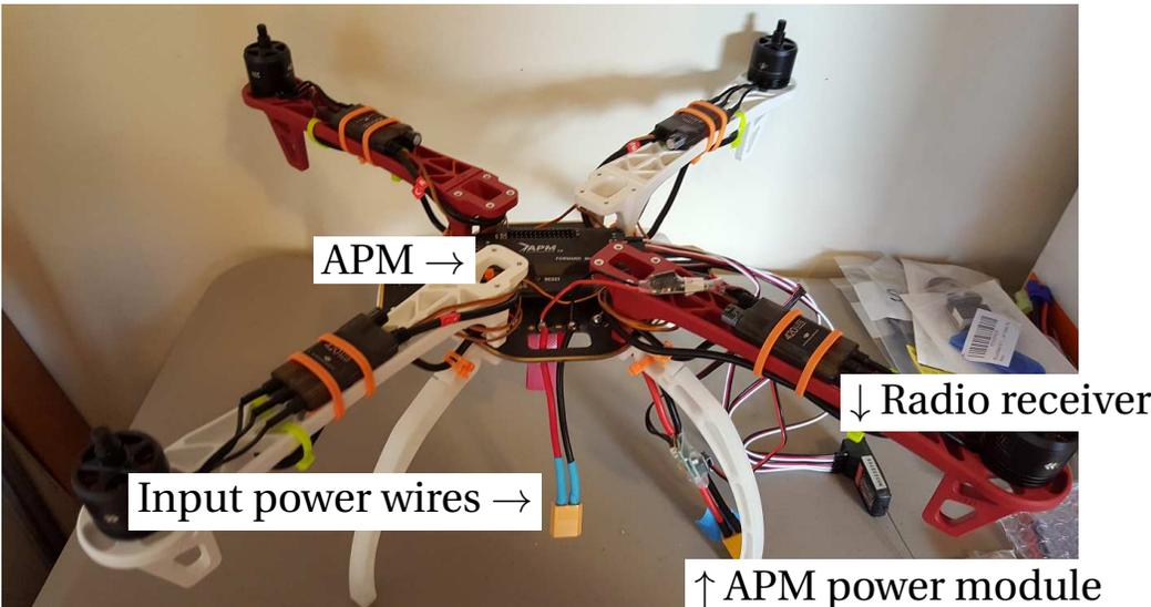
Figure 6: Partial assembly including the APM, radio receiver, power wires, UBEC step down converter, and APM power module
