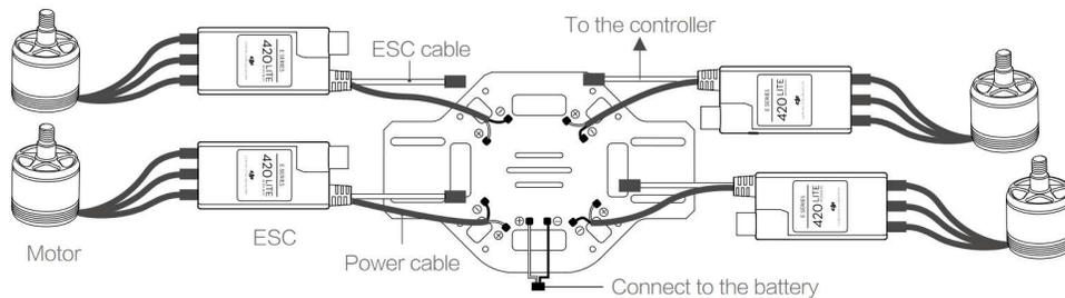
Figure 3: DJI Flamewheel F450 electronic speed controller and motor assembly diagram[7]
