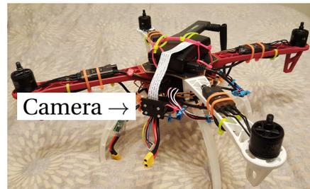
Figure 11: Completed initial drone build without propellers
