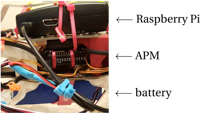
Figure 8: Raspberry Pi, APM, and battery placement
