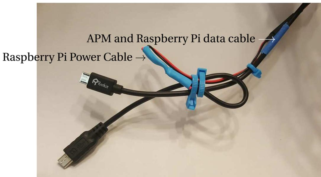
Figure 9: USB cable wiring
