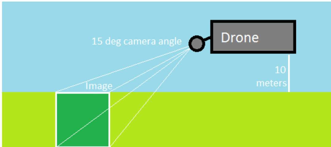
Figure 31: Illustration of drone at 10m, with camera at a 15 degree angle
