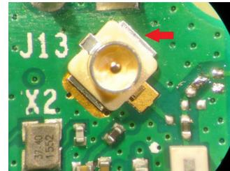
Figure 15: U.FL connector overlaid on the provided pads[45]
