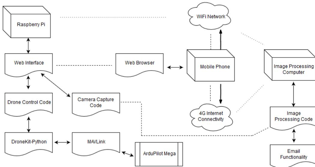
Figure 23: Software Architecture overview, the image processing code is shown in [section 6.](#) and [section 7.](#)
