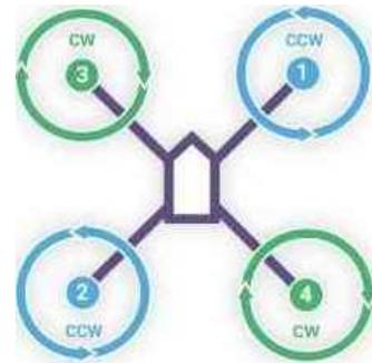
**Figure 5:** Motor channel layout for Quad X configuration[13]
