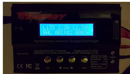
Figure 20: Tenergy TB6-B Balance Charger shown charging a battery.
