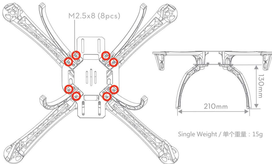
Figure 2: DJI Flamewheel F450 landing gear assembly diagram[9]
