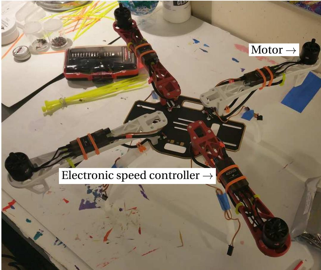
**Figure 4:** Partial assembly of arms, electronic speed controllers, motors, and landing gear
