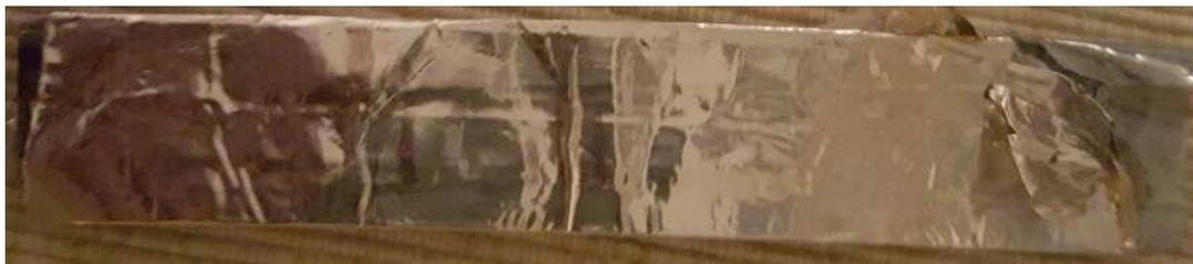
Figure 22: Foil wrapping for camera module ribbon cable
